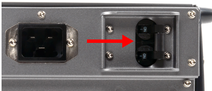
Figure 11 Chassis circuit breaker
